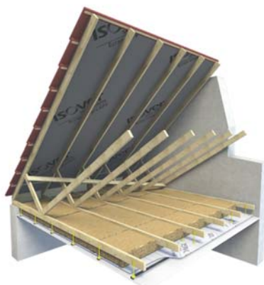
Figure 1 – Installation de l'isolant ISONAT FLEX entre solives
